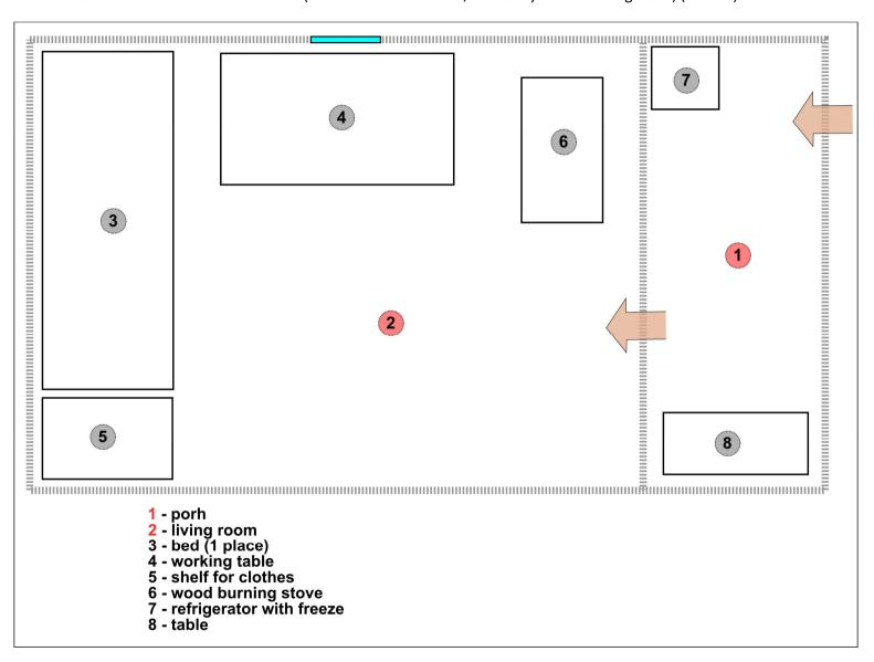
6. Plan of construction of **watch man house** (one room with one bed, heated by wood burning stove) (4 x 4 m).
