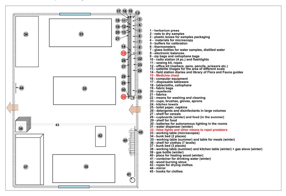
3. Plan of construction of 2nd room (10 x 5 m.), designed for accommodation and work in summer and winter time (9 bed places); in winter the room could be heated according to needs by wood burning heater.
